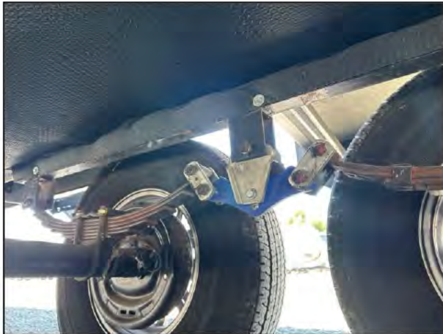
Curbside hanger inside view
