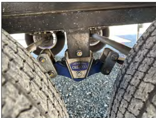
Streetside hanger outside view
