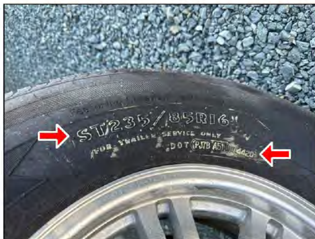
Front Curbside Tire Size and DOT Date
