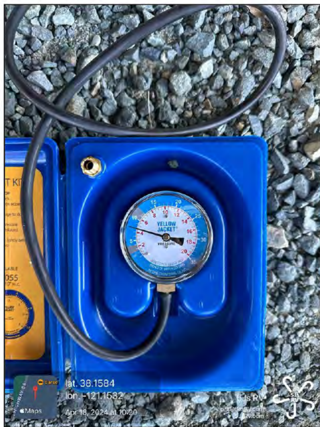
LP Drop Test Start at 1020 PDT
