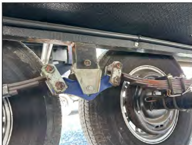
Streetside hanger inside view
