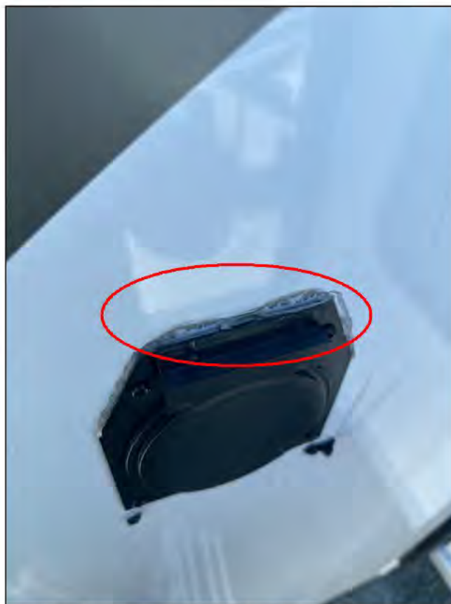
Dryer vent cover at top front of the streetside sidewall (from below)
