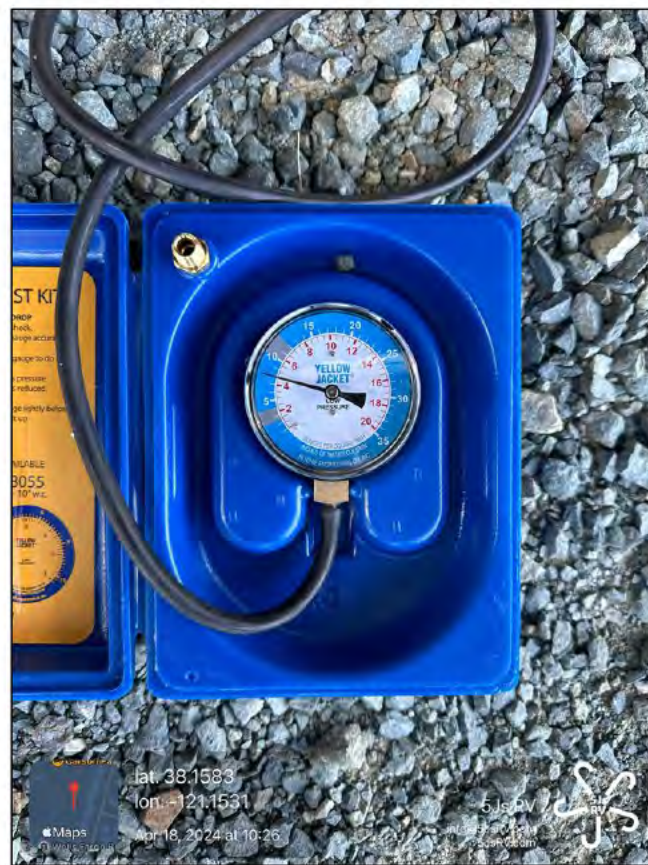
LP Drop Test Finish at 1026 PDT
