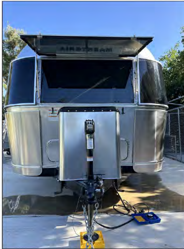
Front wall cap (window open)
