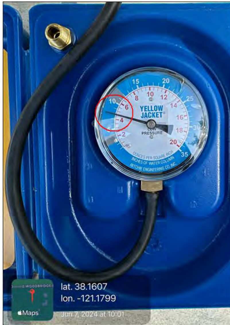
Start of LP drop test at 1001 PDT (8 WCI)
