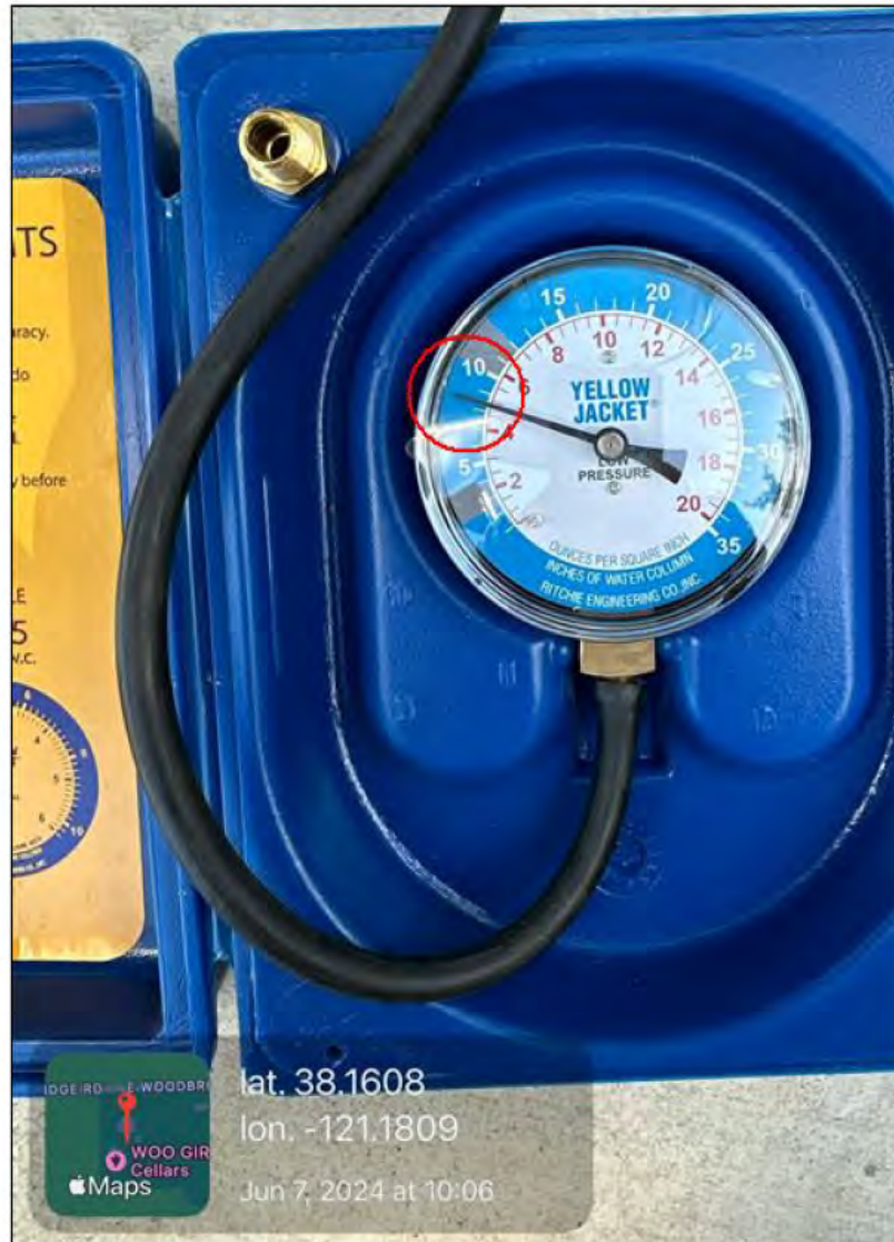
End of drop test at 1006 PDT (8.5 WCI)
