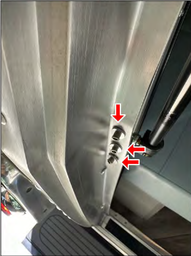
Streetside rear door strut (bottom)
