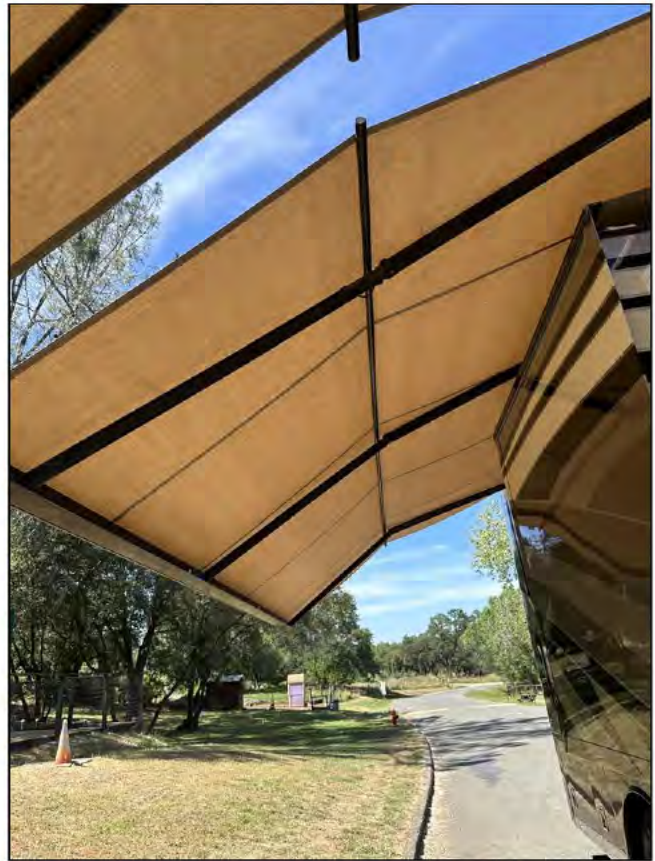
Rear curbside awning (from below)
