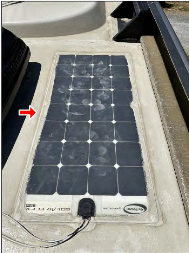
Forward curbside solar panel (100W)
