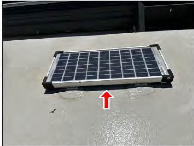
Rear-most streetside solar panel (10W)
