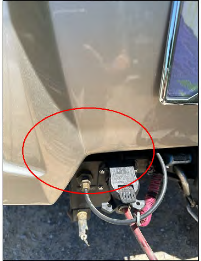
Hairline cracks above air brake line on hitch
