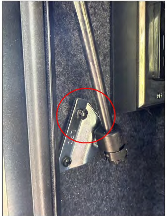
Curbside outdoor TV cargo bay (close-up of rear internal bottom door pneumatic)
