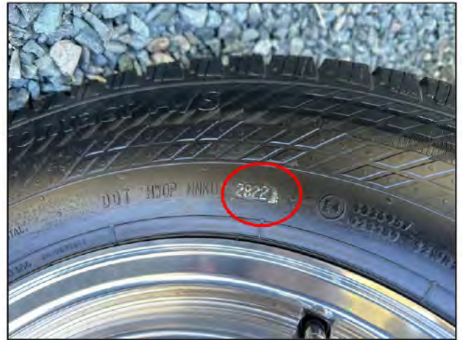
Front curbside tire DOT date
