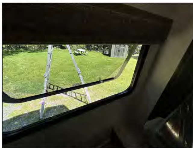
Emergency exit in the rear wall of the rig
